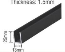
SUC-01 (Black Matt) 'U' Channel (For Fixed Glass) Available in 10 Ft. Thickness: 1.5mm
